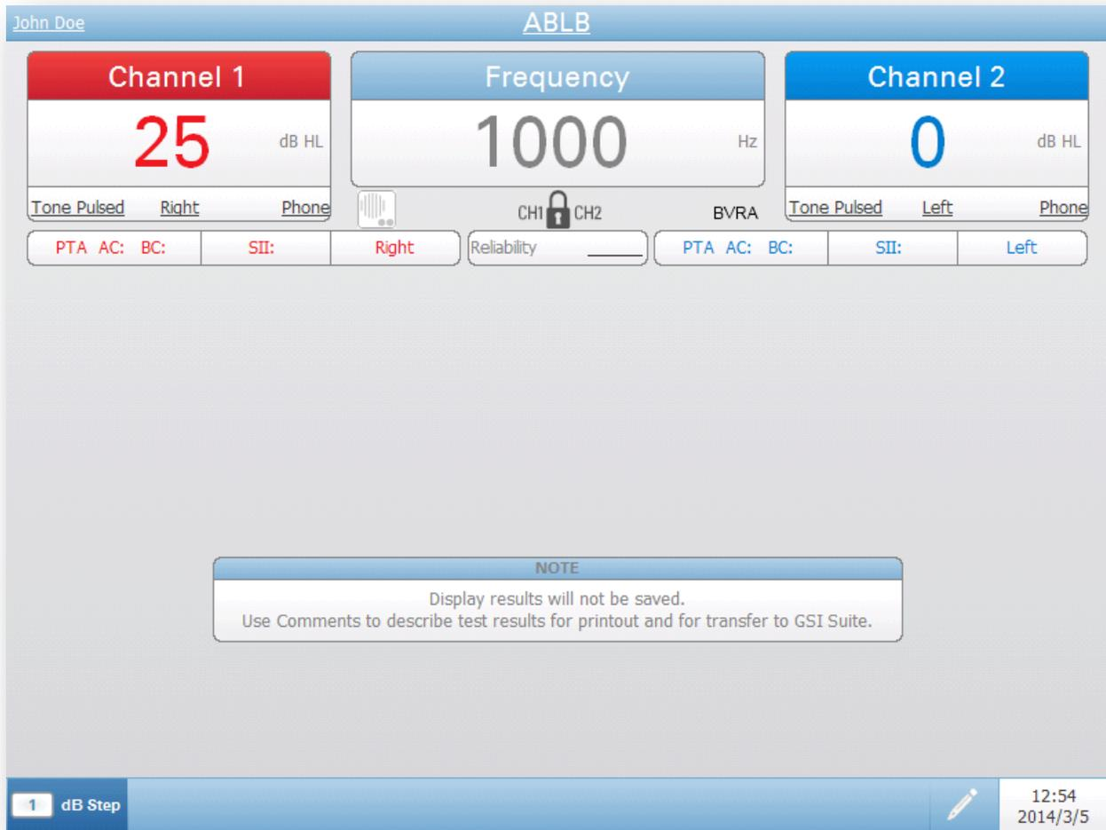
In ABLB (Alternate Binaural Loudness Balance) test the tone is presented alternately between the two ears. The level of the tone stays the same in one ear (i.e. fixed ear) and is varied up / down in the other ear (i.e. variable ear).
