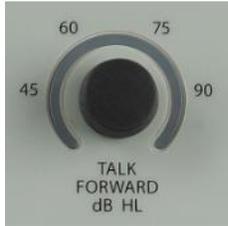
This rotary control allows the operator to adjust the microphone intensity in a continuous range of 45 to 90 dB HL when communicating through Talk Forward.
