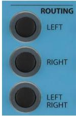
The Routing pushbuttons determine the routing for the stimulus to the output transducer selected for Channel 1 and Channel 2. Left/Right delivers the stimuli from the selected channel to both the left and right transducers with the combined signal. Both the Channel 1 and Channel 2 maximum dB HL limits are appropriately decreased from the non-mixed maximum dB HL limits.
