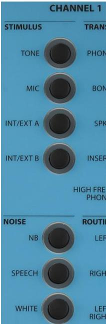
**Tone** — The Tone pushbutton allows the selection of a pure tone stimulus for air/bone conduction testing with the choice of five transducer types.
