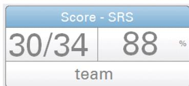
This scoring window displays the speech scores in a percentage value. The scores are populated using the Correct/Incorrect buttons on the front panel of the instrument. The left side indicates the number of correct responses over the total presented. The right side converts this into a percentage. The lower part indicates the current word being presented.
