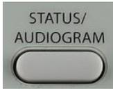
The Status / Audiogram button is used to select the format for the screen display. Pressing it will switch the screen between displaying the Status screen and the Audiogram screen for the Tone, High Frequency, TEN and Speech Test Types. On the Tone and High Frequency test types, this button allows access to the Fine Frequency Resolution option for detailed frequency testing.
