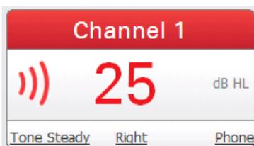
The Channel 1 and 2 windows display the current output for each channel. The sound wave symbol indicates that a stimulus is being presented. This sound wave will be present as long as the present bar is depressed, will flash to indicate a pulsed stimulus, and will be steady if “interrupt” is in the on position. The intensity of the stimulus will be displayed in the color of the ear that has been
