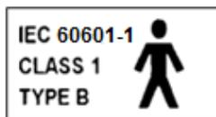
This icon indicates that the GSI AudioStar Pro is in compliance with Class 1, Type B requirements of IEC 60601-1.
