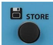
The Store pushbutton, when pressed, saves the current dB HL level representing the current data point (threshold level, MCL, UCL, tinnitus, aided sound field, cochlear implant and effective masking level if selected, as well as transducers and routing. Pressing Store in the Speech testing mode will save the current test type, word list, score and other applicable speech data. In the Display Audiogram format, the appropriate symbol appears each time the Store button is pressed.
