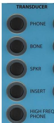
The Transducer pushbuttons allow the easy selection of the transducer for each stimulus available for Channel 1 and Channel 2. A transducer selection may be changed at anytime.
