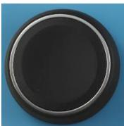
The GSI AudioStar Pro contains two independent HL rotary controls for test signal and masking intensity level control with a range of -10 dB HL to 120 dB. HL Maximum dB HL values apply to the mid-frequencies with earphones only. Refer to the specific transducer for dB HL limits in the Table in Appendix 1.
