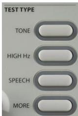
Test Type buttons allow the operator transition between audiometric evaluation components with a single button press. Pressing a test type button loads all stimuli, routing and transducer preferences from default settings or from customized protocols determined in the Config App. Test types are pre-programmed to optimize efficiency and workflow.
