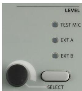
**Test Mic, Input A and Input B Level Controls** — To calibrate the test signal for the test microphone or the external devices, use the Select button to activate the LED associated with the device. Then use the rotary knob to adjust the signal intensity until an indication of 0 dB on average is obtained on the selected channel VU meter.
